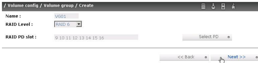
Figure H.2: choose RAID level and disks.
